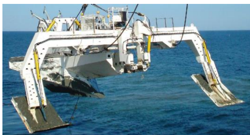
Pipeline Burial Plough (Bisso Marine, 2016).
