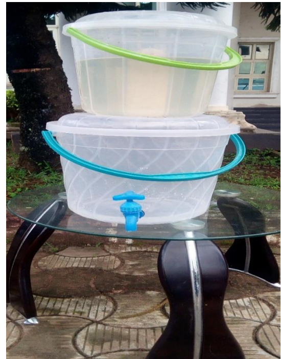
Figure 2: Water Filtration setup using produced ceramic candle filter
