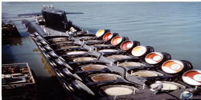
Fig 65: USS Sam Rayburn: hatches for her Polaris missiles 273 Fig 66: A Russian Project 941 (Typhoon class) SSBN 274
