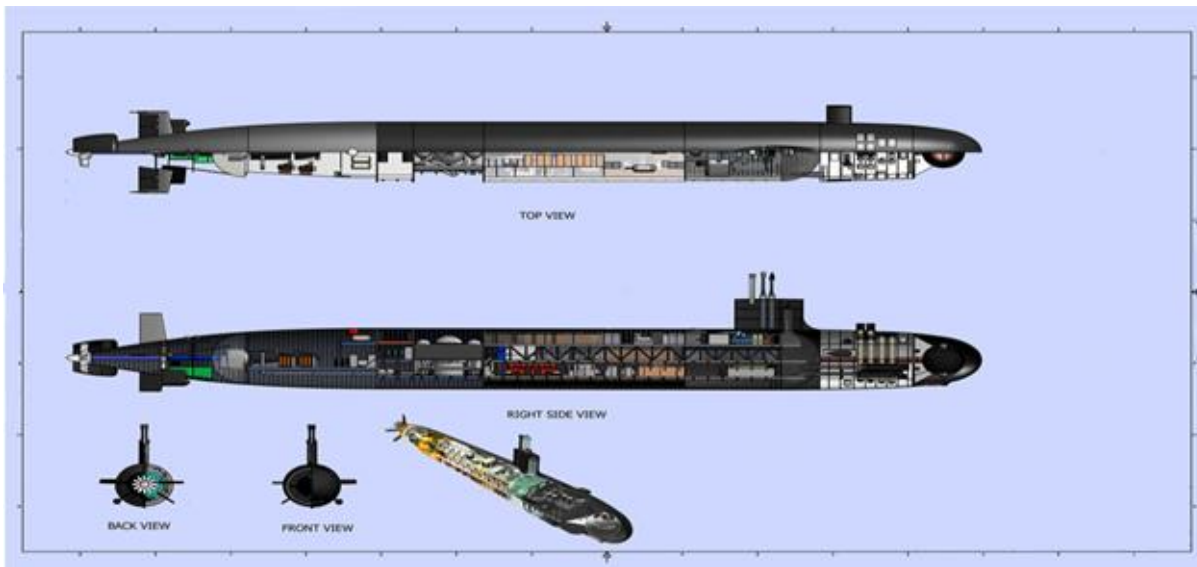
Fig 72: US Navy Virginia Class nuclear submarine with single hull design 302
