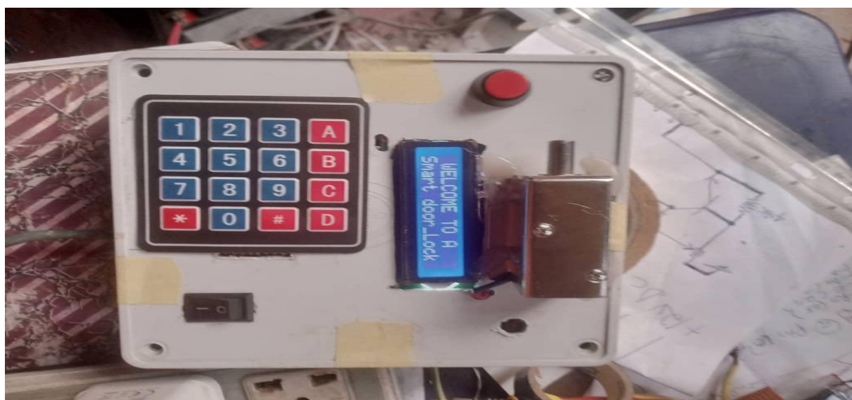
Plate 4.2: A Smart door lock system showing power up state
