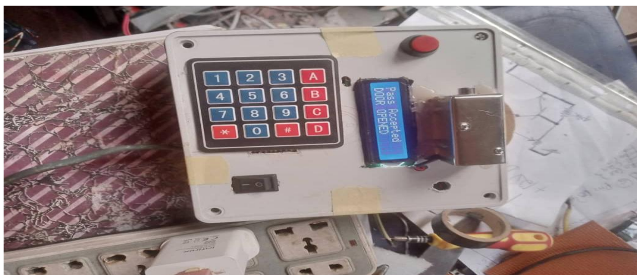
Plate 4.3: The smart door lock in operation showing access granted
