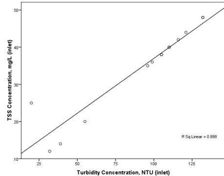
Fig.11 Correlation of Turbidity Concentration at Inlet with TSS Concentration at Inlet
