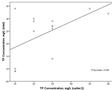
Fig.14 Correlation of TP Concentration at inlet with TP Concentration at Outlet 2
