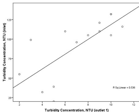
Fig.9 Correlation of Turbidity Concentration at Inlet with Turbidity Concentration at Outlet 1
