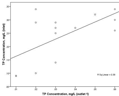
Fig.13 Correlation of TP Concentration at Inlet with TP Concentration at Outlet 1
