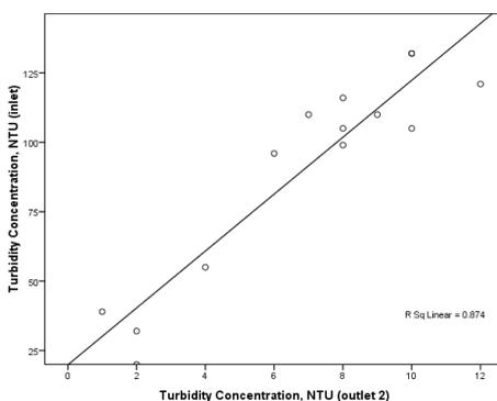
Fig.10 Correlation of Turbidity Concentration at Inlet with Turbidity Concentration at Outlet 2
