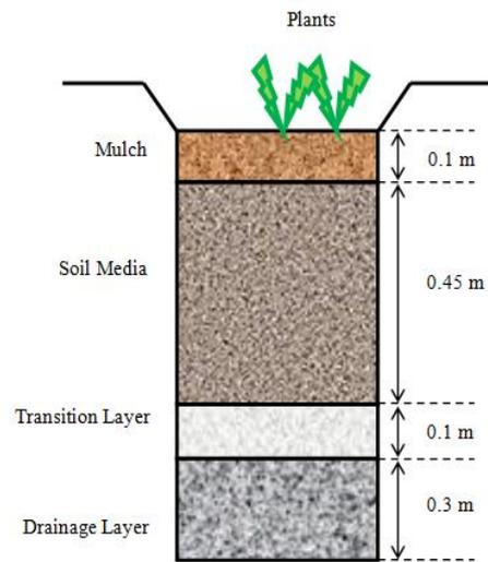
Fig. 2 Cross Section of Bioretention 2
