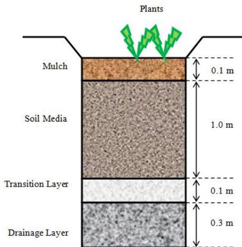
Fig. 1 Cross Section of Bioretention 1
